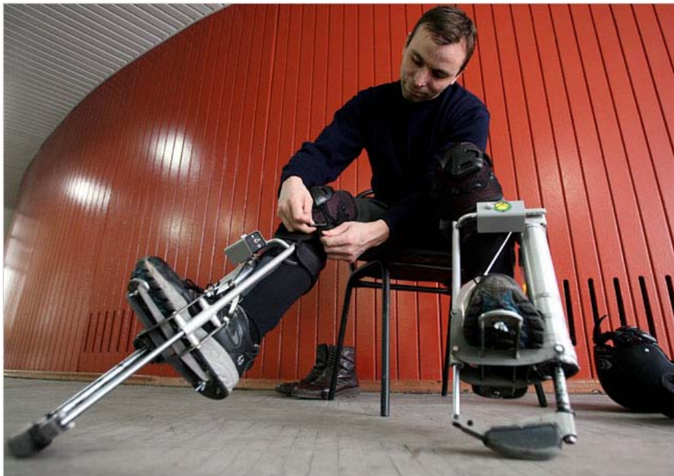
Figure 3-3. Boots powered by internal combustion and created by an independent inventor, Russian engine designer Viktor Gordeyev. (Source: Joseph Sywenkyj/Redux)
